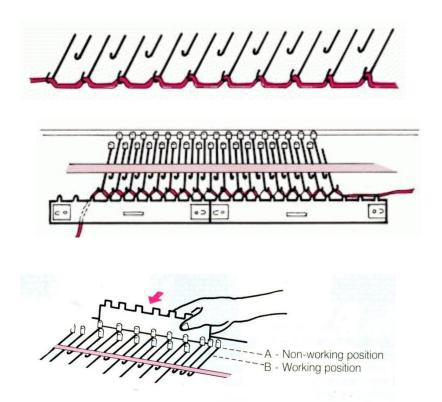
The yarn is hooked on each needle in position B and needles in position A do not knit.
